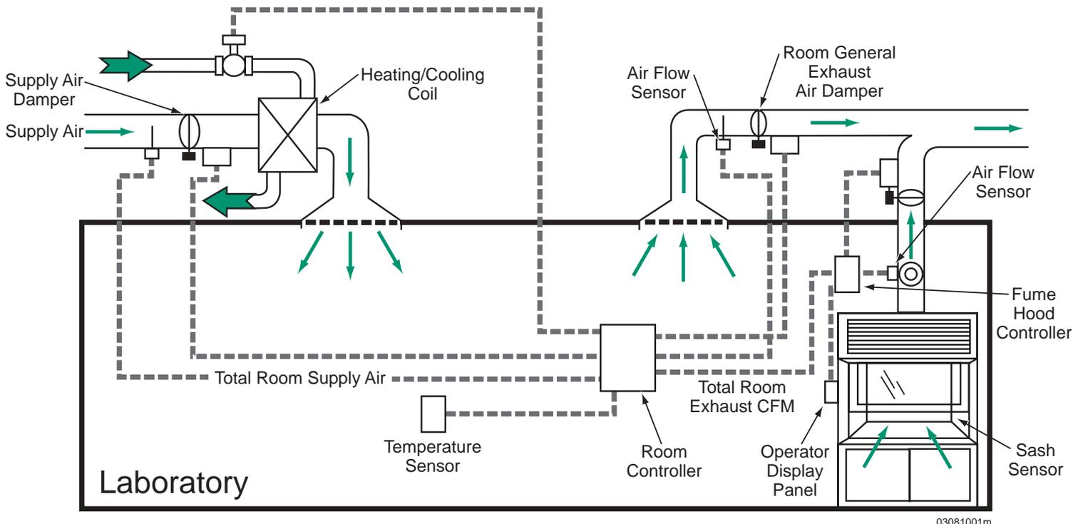
Figure 4. VAV laboratory control system (information courtesy of Siemens Building Technologies, Inc., and CAC, Inc., the PETL system installing contractor)
