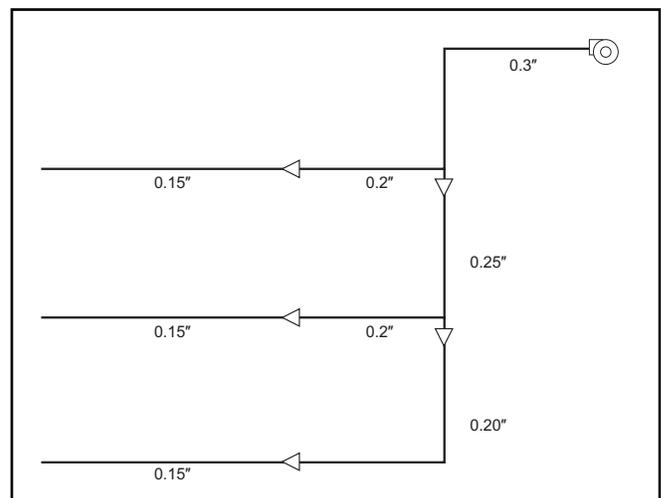
Figure 3. Example of duct sizing using the friction rate reduction method (Hydeman et al., 2003, p. 90).
