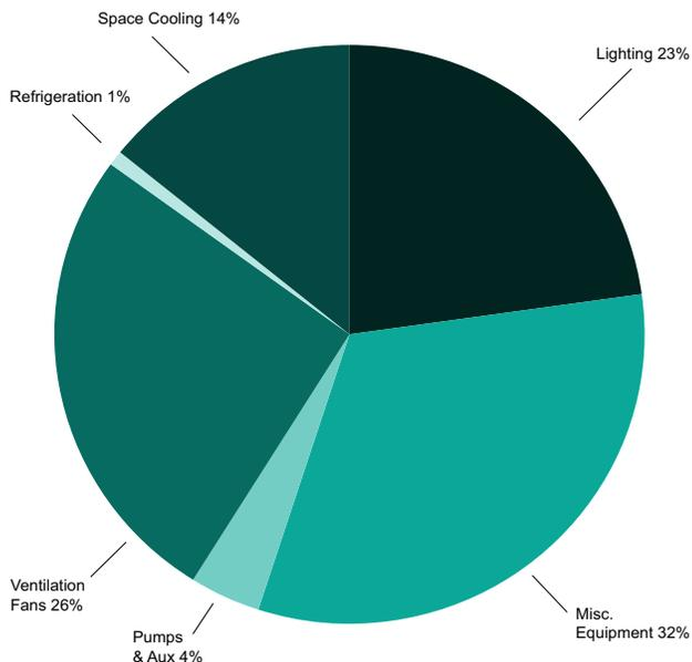
Figure 1. Fan energy has a major impact on labs’ electricity use. Data courtesy of CannonDesign, 2013.
