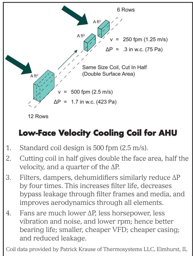
Figure 2. Coil configuration for low face velocity.
