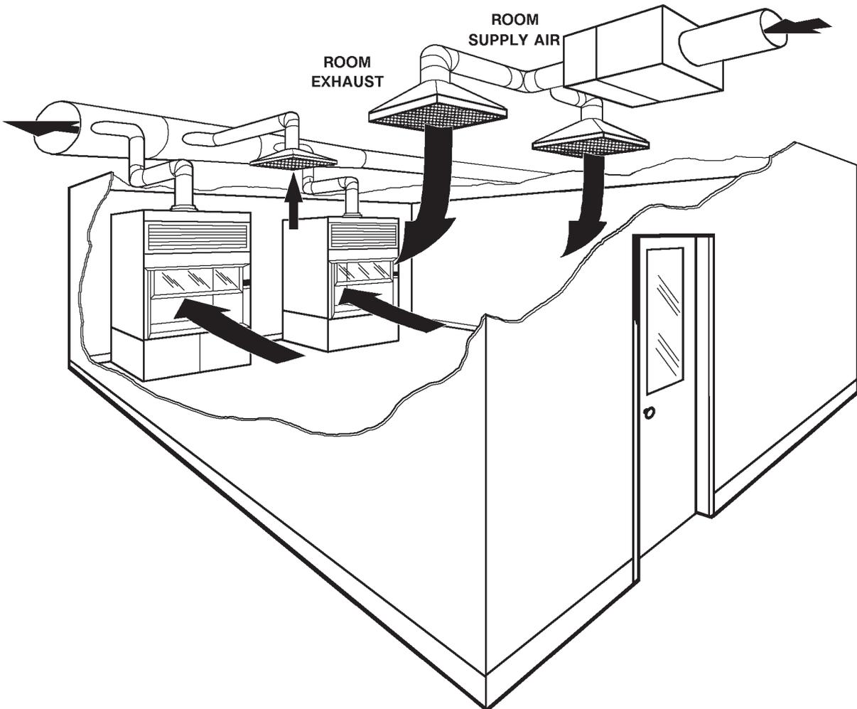
Figure 4. Room pressurization physics, illustrating a lab that is negatively pressurized compared with the space outside of it. Source: Siemens.
