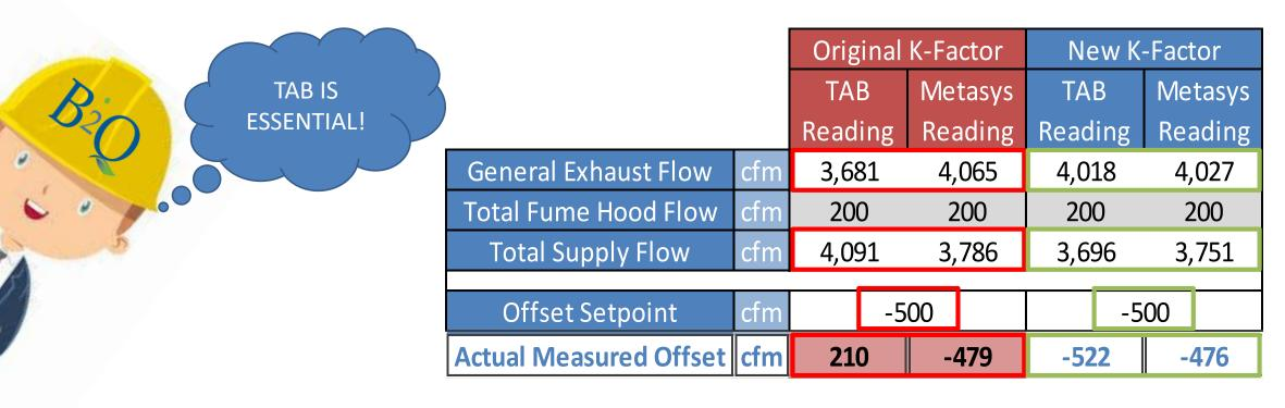
A K-Factor (or pickup gain) relates pressure velocity and area to airflow in VAVs (and other flow applications)
