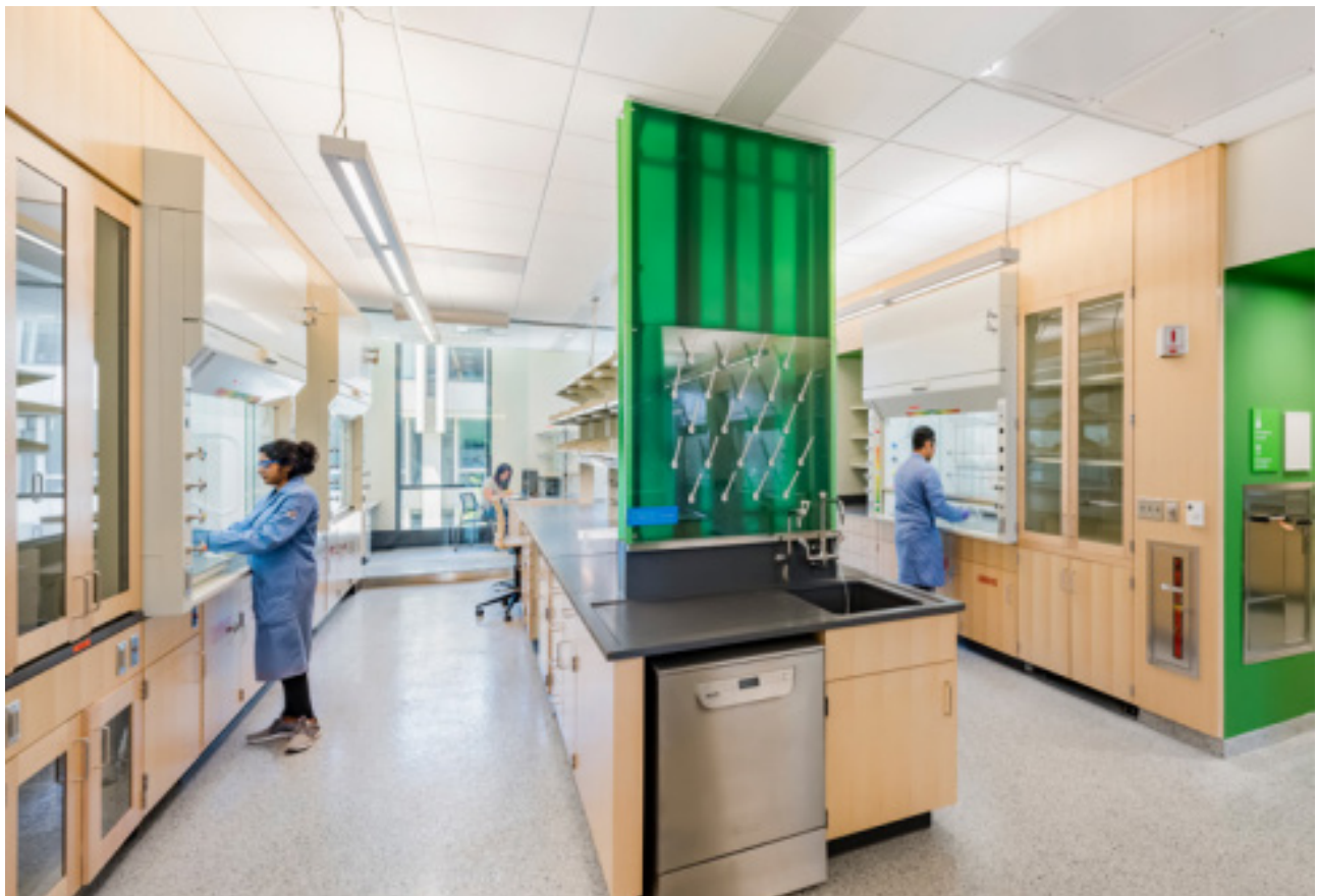
Figure 8. The designers of the Life Science Laboratories at UMass Amherst placed office cubicles next to the vertical fenestration to take advantage of direct daylight from perimeter glazing. HLB Lighting’s design seamlessly merges daylight and artificial lighting in the writeup and lab spaces. The work desk placed parallel to the double-height windows, followed by lab stations, promotes daylight integration in the space. Source: HLB.
