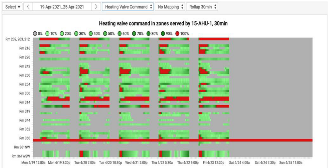
Figure 3. Sample data analytics and visualization tool used by the LBNL ongoing commissioning team. This tool shows the zone reheat valve commands for all zones served by a selected air-handling unit (y axis: zones) over a week (x axis: time) and allows the user to identify patterns and outliers. Here, one zone has its reheat valve 100% open all the time, shown as a solid horizontal red bar. Source: Berkeley Lab.
