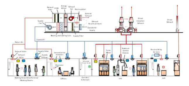
Figure 2. Diagram of Airflow Systems serving different types of Indoor Environments
