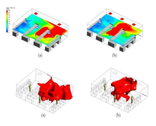
Figure 5.Distribution of contaminant concentration at the breathing zone after 720 s of release of contaminant for a typical laboratory setup with two and three exhaust grilles shows location and number of exhaust grilles can significantly impact the ventilation effectiveness. (CFD analysis is performed by AnSight LLC, Ann Arbor, MI, USA.)
