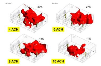
Figure 4. Cloud of 25 ppm concentration showing the spread after 720s release of contaminant shows contaminant spread is a volumetric phenomenon. Increasing ACH would help in minimizing the Spread Index, however, the location of the highest concentration depends on several HVAC related factors. (CFD analysis is performed by AnSight LLC, Ann Arbor, MI, USA.)
