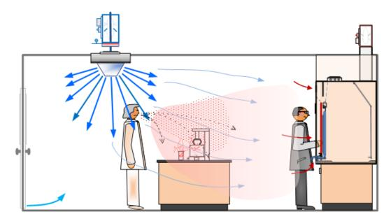
*Figure 6. Diagram of laboratory with ventilation system that maximizes dilution and removal of contaminant to reduce exposure dose.*
