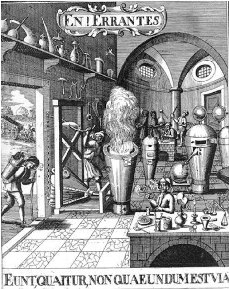
We can call it an early high temperature laboratory and the heating systems did well advance. The man in the door brings new wood and charcoal to the furnaces equipped with air bellows to reach higher temperatures in the ovens. Ventilation of the room is still done by open doors and windows, but the room is much higher and has openings here allowing fumes and gases to evade. The picture shows a lot of amusing details such as smoking was permitted in the labs of this time.
