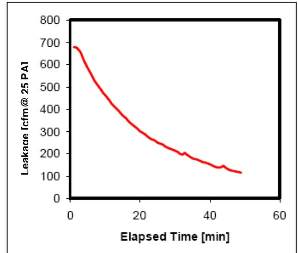
Figure 3: Example sealing profile (third floor northwest)
