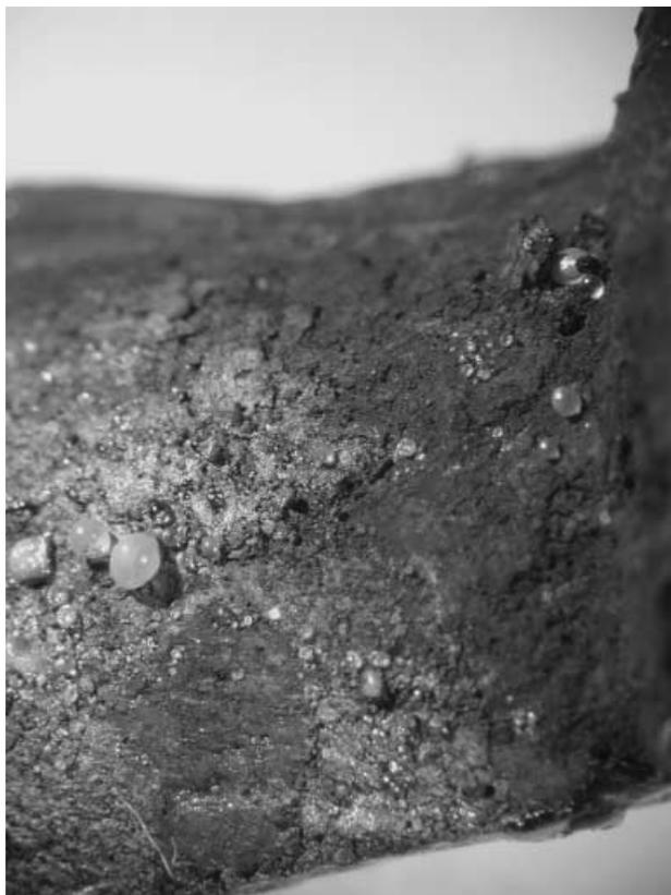
Figure 6. Rivet head from the *Hunley* exposed to the air for only a couple of days: Note initial indication of active corrosion in the form of the weeping phenomenon. (Copyright Friends of The Hunley Inc., 2000)
