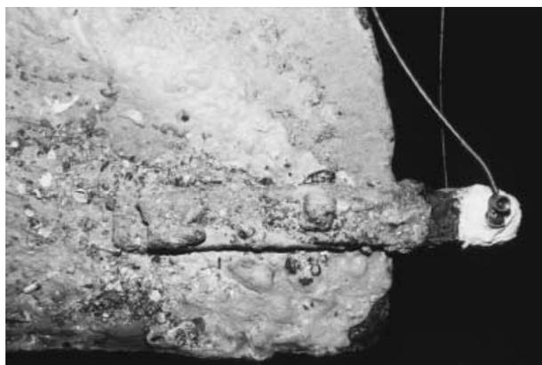
Figure 4. The resistive effect of the riveted seams being negligible, the main connection to the hull was made at the former spar connection using a modified bolt covered with an epoxy coating. (Copyright Friends of The Hunley Inc., 2000)
