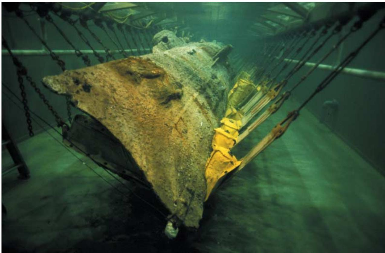
Figure 3. *H.L. Hunley* resting in its tank at the Warren Lasch Conservation Center soon after its recovery. Note the anodes in the white perforated pipes parallel to the hull. (Copyright Friends of The Hunley Inc., 2001)
