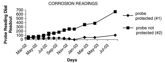
Figure 8. Probe corrosion readings.
