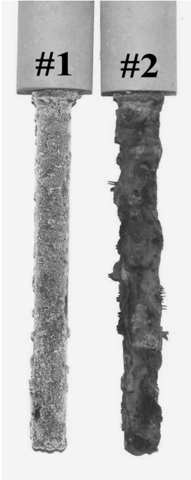
Figure 7. Photograph of mild steel test probes taken on August 27, 2003. (Copyright Friends of The Hunley Inc., 2003)
