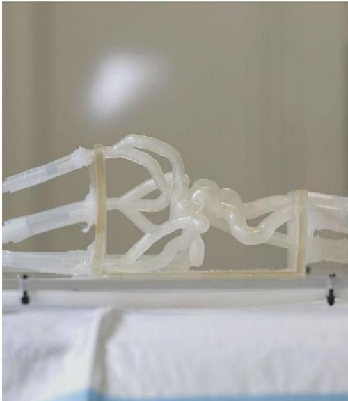
*Caption: This 3D Printed vascular model is used for training and testing with blood clots. Printed on a Stratasys 3D Printer. Credit: The Jacob's Institute*
